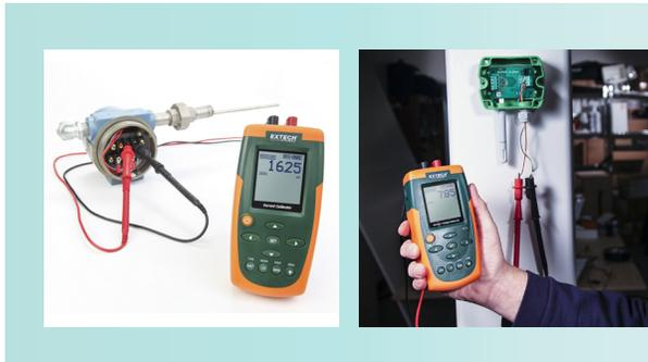
**Precision "source" for calibrating process devices.**
